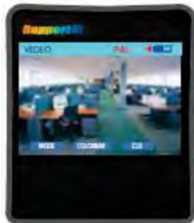
CCTV Field Monitor
